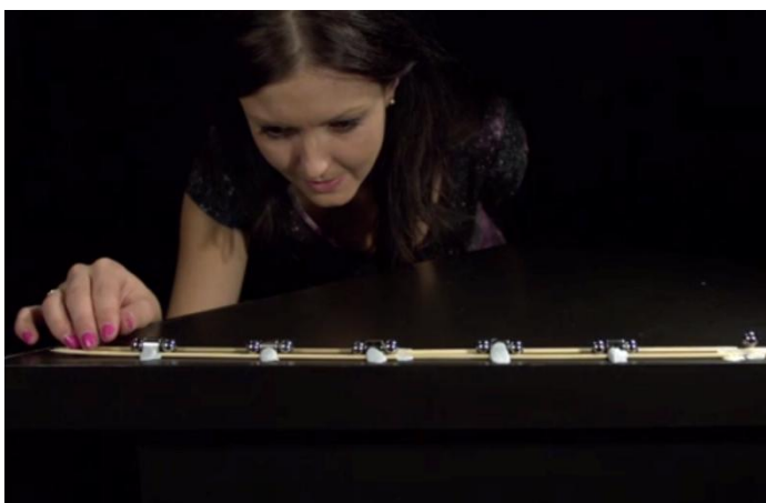
Figure 1: The magnetic rocket. Using skewers, ball bearings, magnets and blu-tack.
