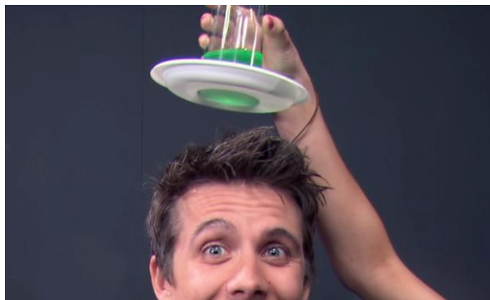
Figure 2: Levitating plate? The plate is held against the glass by the surrounding air pressure.
