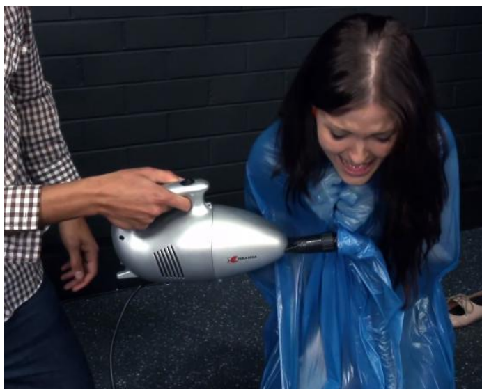
Figure 1: Vacuum sealing by removing air. The pressure from the surrounding air squeezes the bag and its contents.
