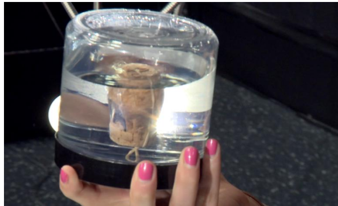
Figure 2: Homemade accelerometer. This object simulates the action within the utricle.
